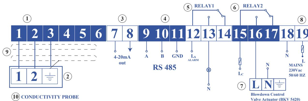
Figure 12 : BK 5000-T Wiring Diagram with BD 5400
