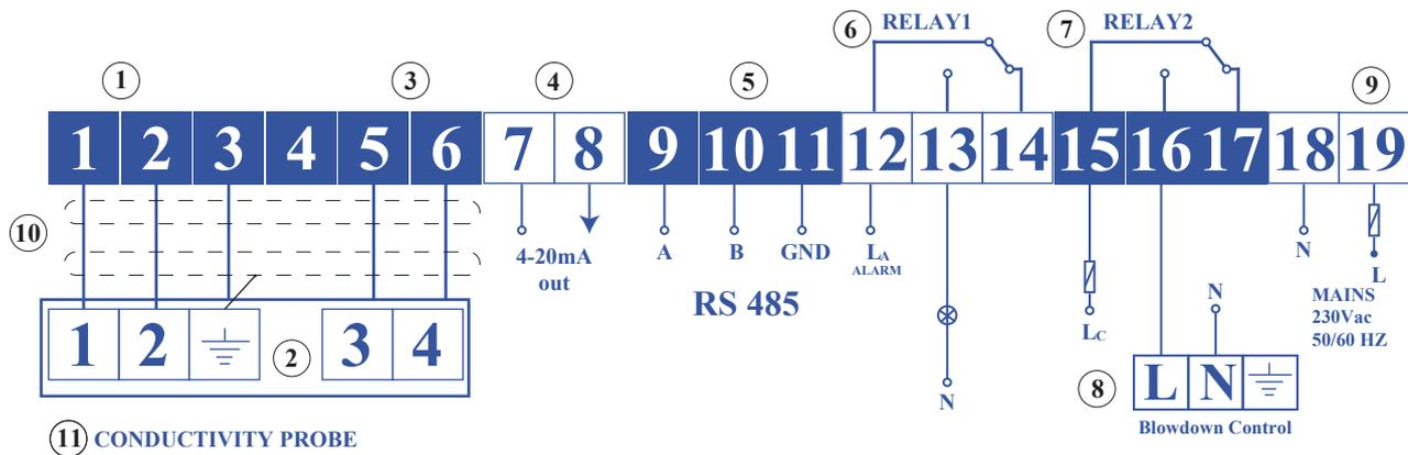
Figure 11 : BK 5000-T Wiring Diagram with BD 5600-T & BD 5300-T
