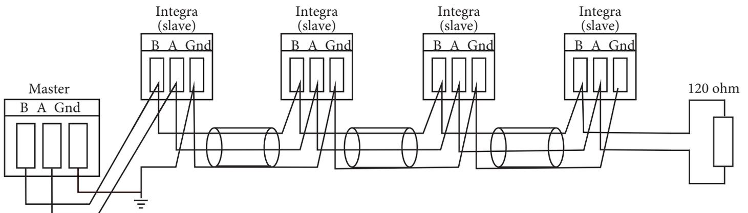
Figure 40 :Wiring Topology
