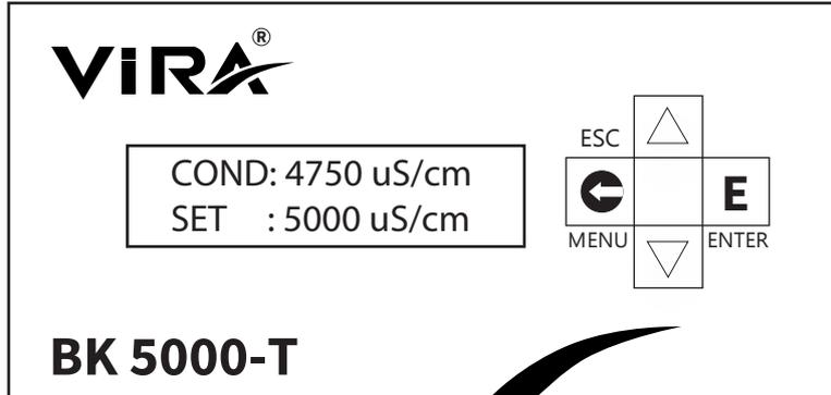
Figure 15 :Front Panel and Button Functions
