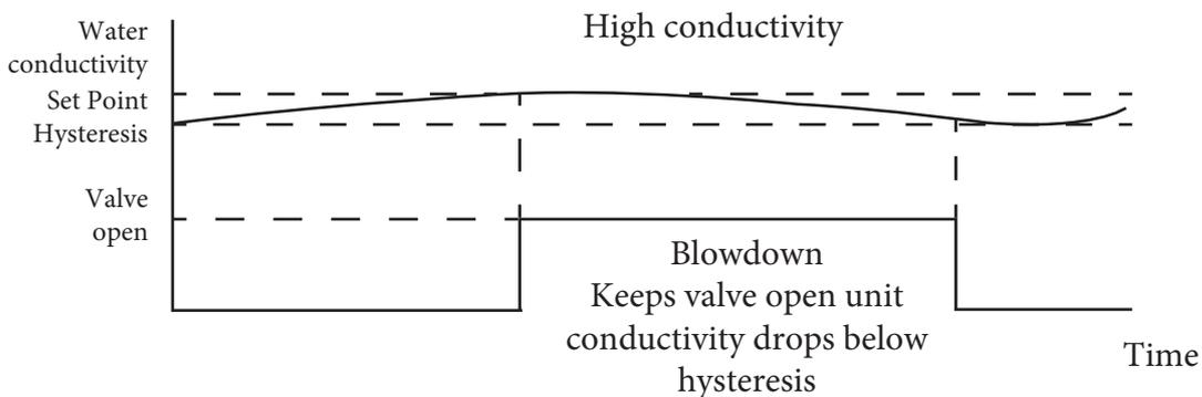
**Figure 1 :** Automatic Blowdown vs Time
