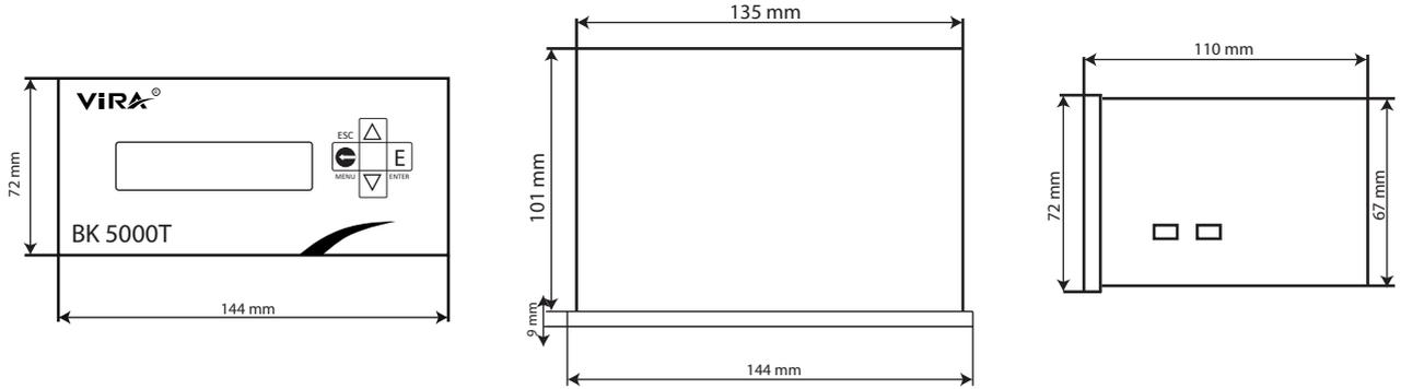
Figure 8 : Conductivity Controller Dimensions
