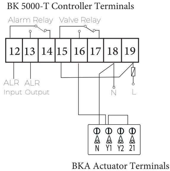
**Figure 13 :** Wiring between BK 5000-T and BKA Actuator
