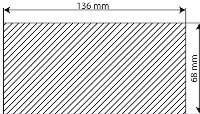
Figure 9 : Panel cut out dimensions of Conductivity controller BK 5000-T
