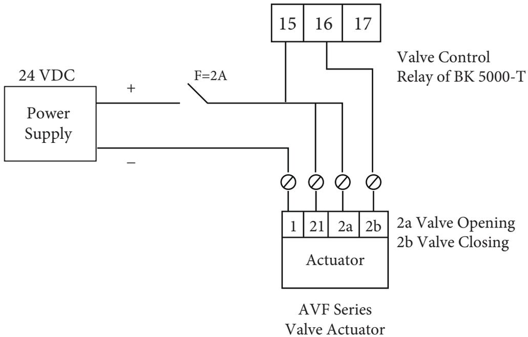
**Figure 14 :** Wiring between BK 5000-T and AVF Actuator
